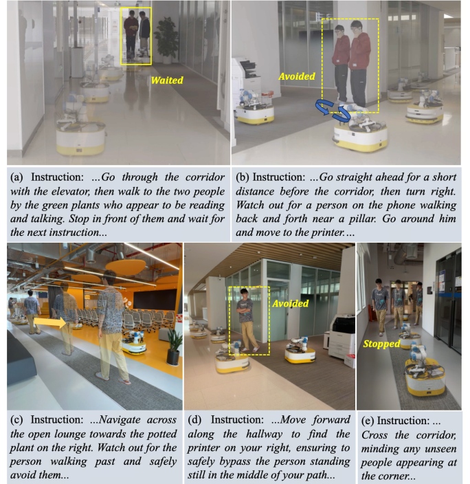
Fig. 7. Qualitative results of real-world deployment on the NXROBO Leo platform. (a) Semantic reasoning enables the agent to approach and wait for interacting pedestrians. (b) Geometric forecasting allows proactive detour planning around a pacing person. (c) The agent safely avoids a pedestrian crossing its path in an open lounge. (d) It correctly identifies and bypasses a stationary human blocking a hallway. (e) It successfully anticipates and yields to an unseen pedestrian appearing from a blind corner.
